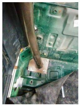
Push the main hoop back until the floor plate is against the rear firewall. Then center the bar side to side. Once in place drill one hole in each floor plate at the bottom of the main hoop.
